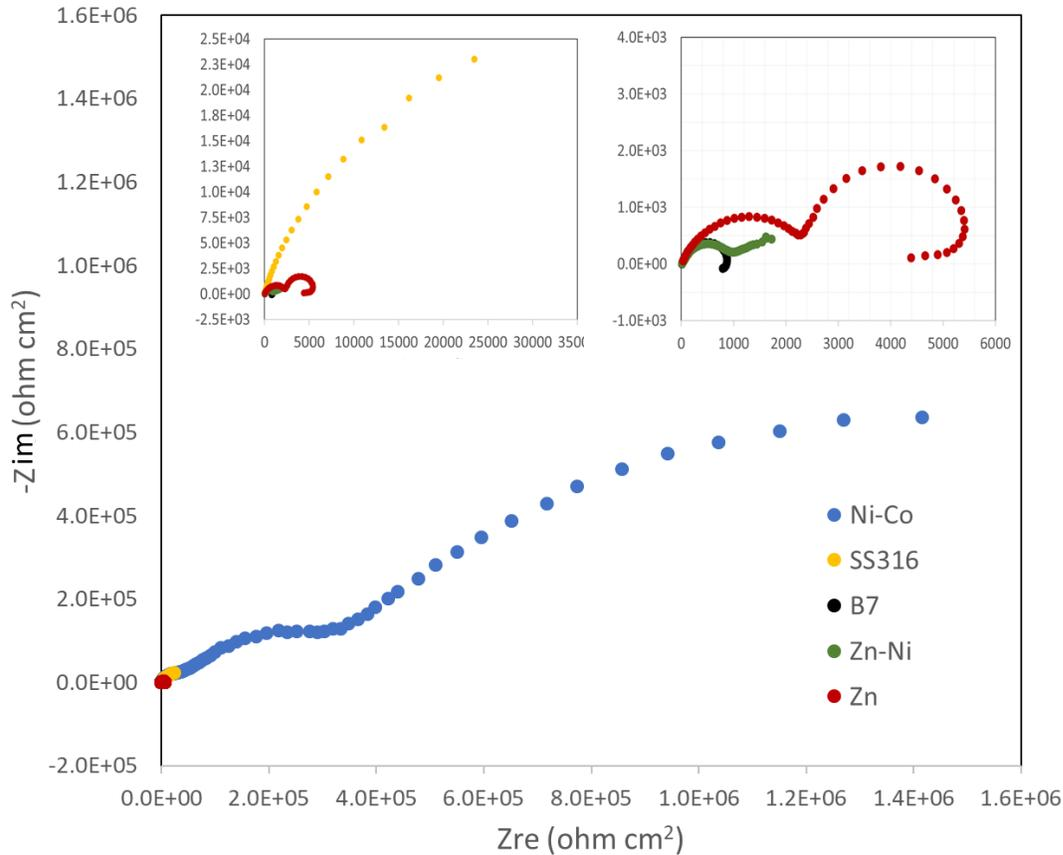
**Figure 1. EIS data for Ni-Co, SS316, AISI 4140 (B7), Zn-Ni, and Zn in 3.5wt% NaCl.**
