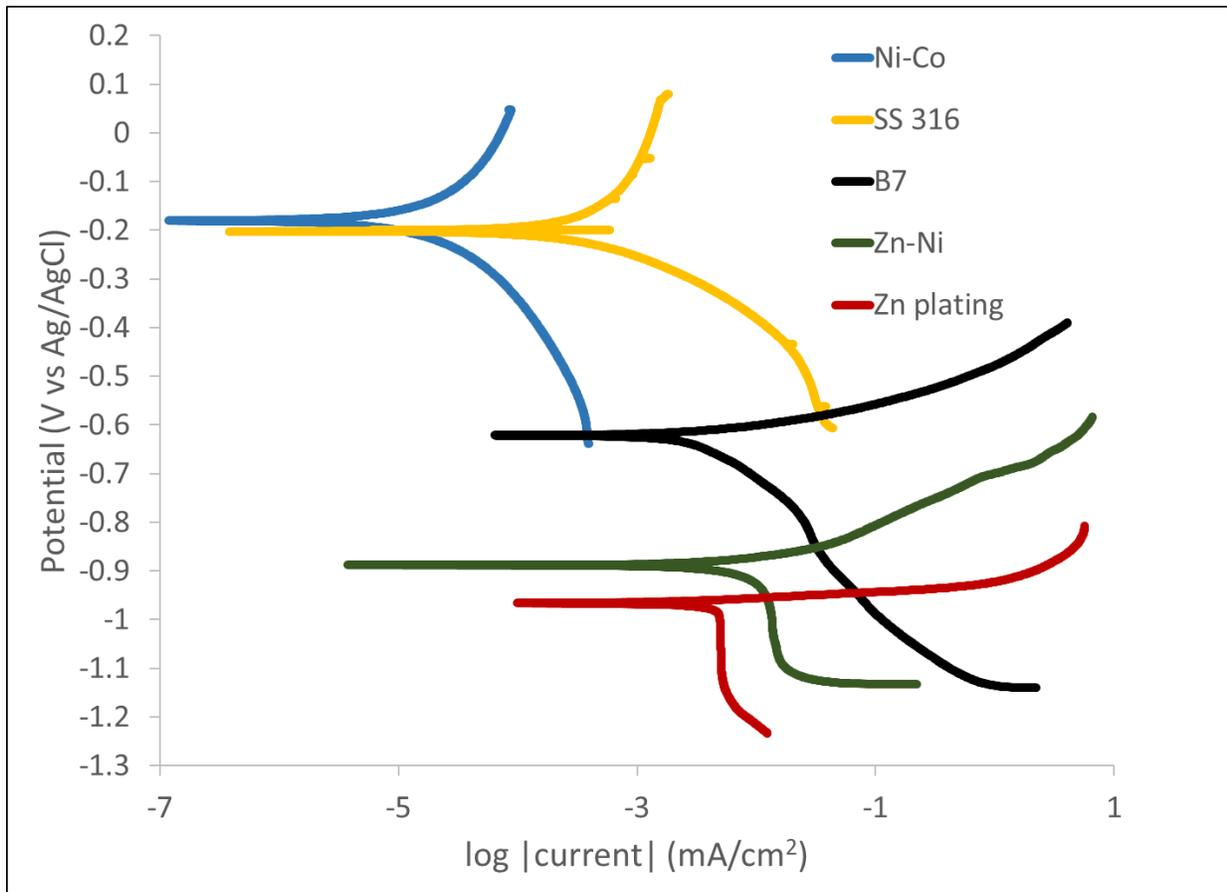
Figure 2. Potentiodynamic plots for Ni-Co, SS316, AISI 4140 (B7), Zn-Ni, and Zn exposed to 3.5wt% NaCl.
